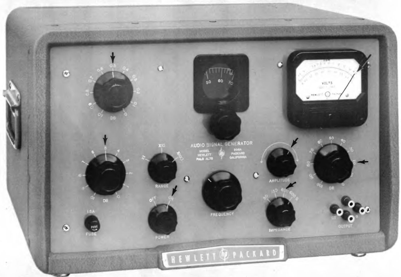
Fig. 2. Model 206A Control Panel Dial Settings for Generator Output of .23 Volts Across 600 Ohms
